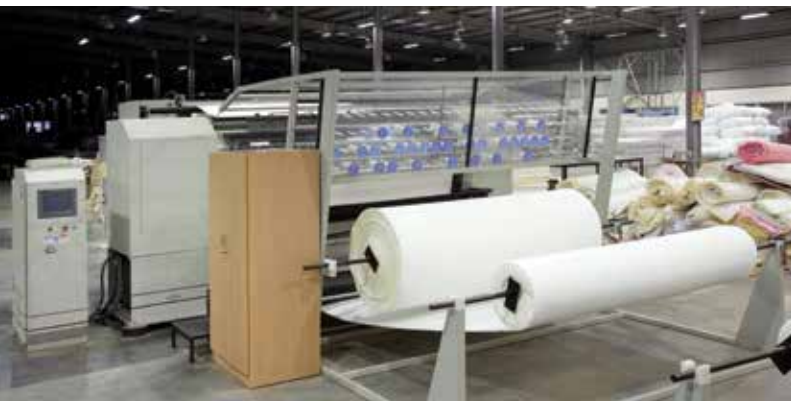
Foam is readied in varying thickness before being stapled on to a spring-and-coil shell
