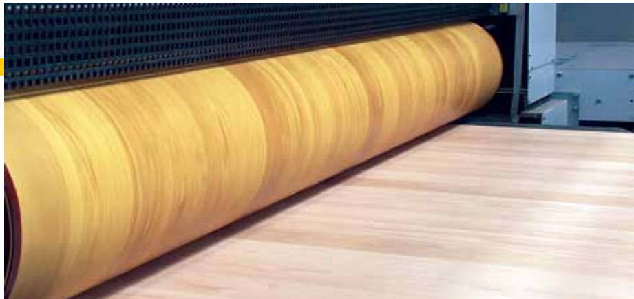
The first of three application roller of the Wemhoner Masterline direct printing plant installed in Turkey
